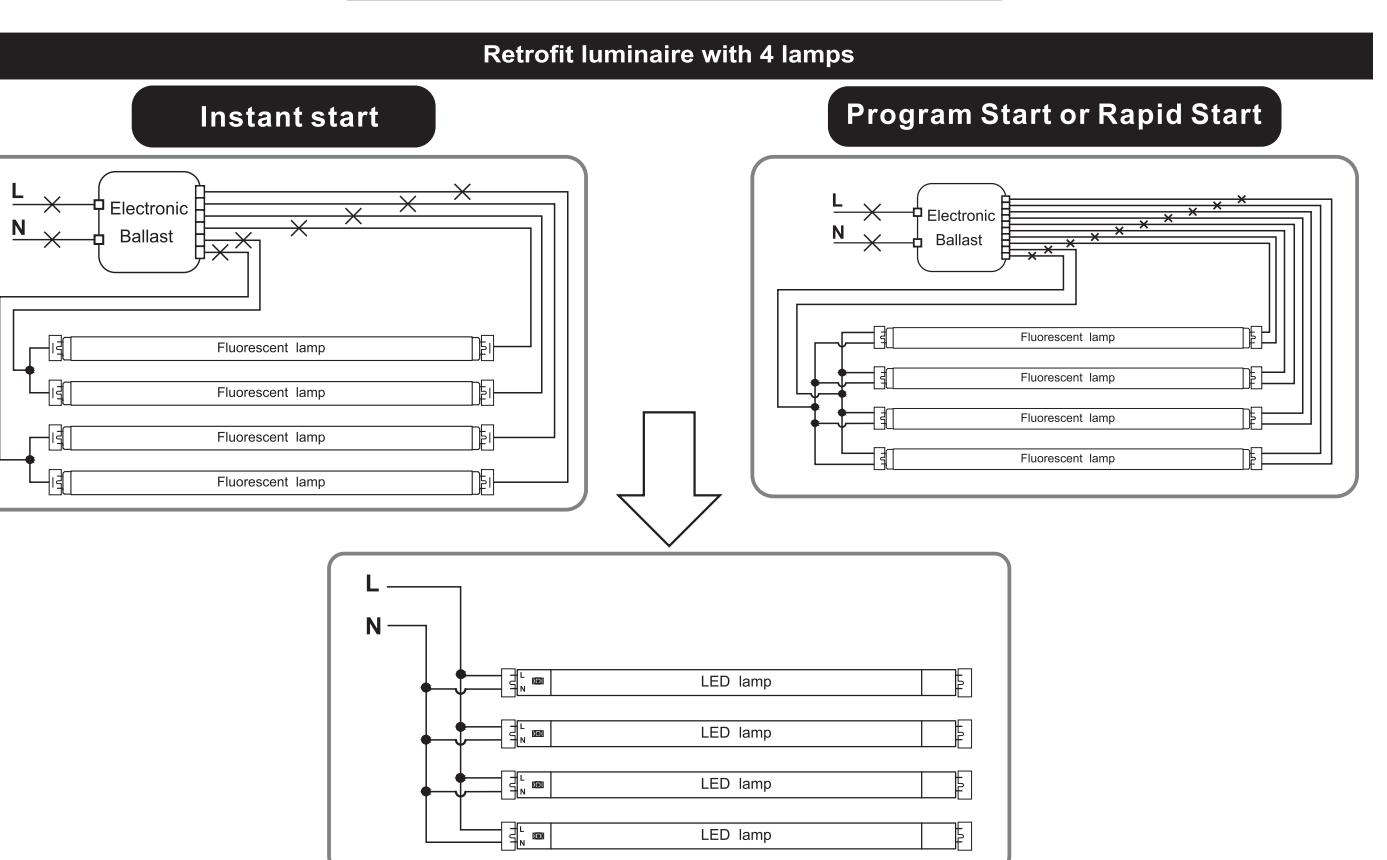
**⚠ The below ballast wiring represents typical configuration. The actual ballast wiring varies according to ballast model. It is not needed to change socket (if in good condition) to operate double ended lamps, regardless the type of sockets. Please make sure one side of fixture is connected to Live (L) and the other side to Neutral (N).**
